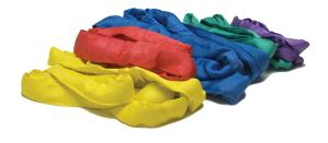
Polyester round slings have a continuous loop of polyester yarn covered by a double wall tubular polyester jacket. Slings are color coded by rated capacity fo easy identification. Light weight and flexible for easy rigging. Very low stretch, good for close quarters lifts. Resists moisture absorption, rot, milldew and most industrial acids and bleach. Soft seamless cover protects and grips the load. Cover protects core yarn form UV degradation.
